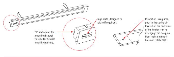
The heater is drilled and threaded for standard 1/2" conduit fittings. The installing electrician will need to provide the appropriate rigid metallic, flexible or liquid tight conduit for the installation location.
