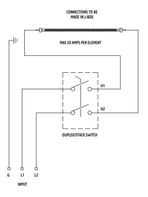
Decora Switch DPST Double Pole Single Throw Range:120/277 VAC Recommended not to Exceed 120 VAC = 1800 Watts Max 208/220 VAC = 3000 Watts Max 240/277 VAC = 4000 Watts Max 20 Amps Max
