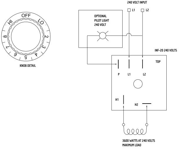
Mechanical Bi-Metal Operation Double Pole Single Throw (DPST) snap action 240 VAC 3600 watts max 15 amps max
